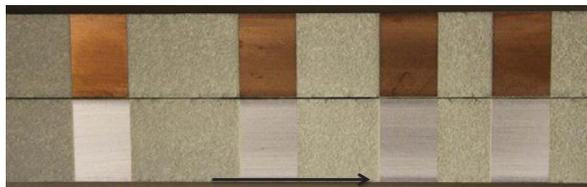
Fig. 5. Failure surfaces of specimen C, suggesting interfacial failures in copper covered regions.
