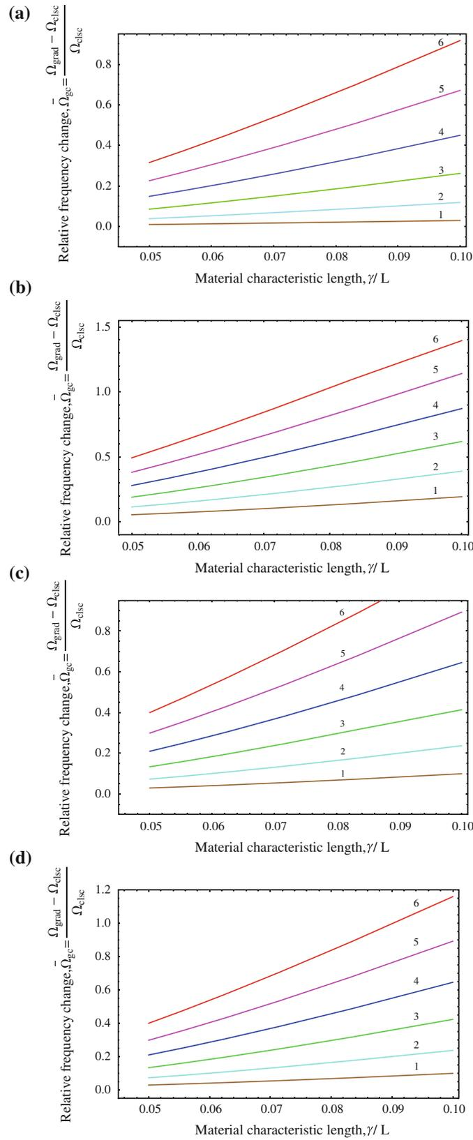
**Fig. 1** Dependence of the relative frequency change upon the non-dimensional characteristic length for a beam with **a** both ends clamped, **b** cantilever, **c** clamped-simply supported, and **d** simply supported. A number on a curve represents the frequency (1st, 2nd, . . .) for which it is plotted
