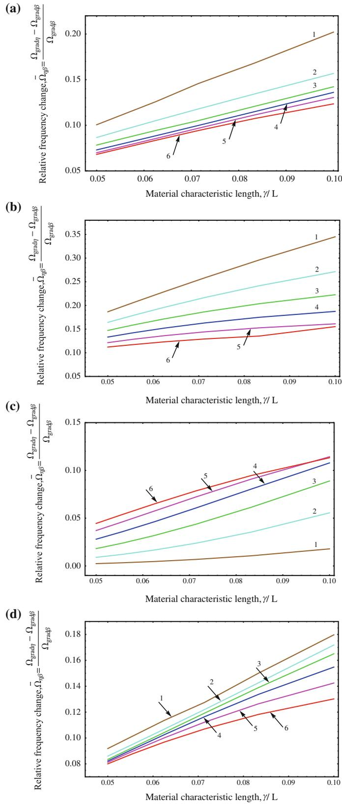
**Fig. 2** Dependence of the relative frequency change for two types of higher-order boundary conditions; **a** clamped–clamped beam, **b** cantilever, **c** clamped–simply supported, and **d** simply supported. A number on a curve corresponds to the frequency for which the plot is shown
