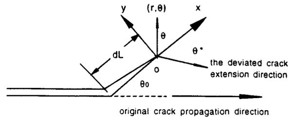
Fig. 1 Deviated semi-infinite propagating crack tip
