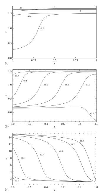
Figure 4. (a) Spatial distribution of the nondimensional shear stress at times 0, 20, 40, 60.4 and 60.7 µs; spatial distribution of (b) the shear stress and (c) the velocity at different times during the localization phenomenon. Curves are plotted at 0.2 µs interval.
