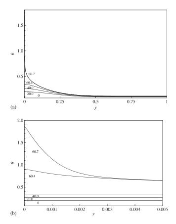
Figure 5. Spatial distribution of the nondimensional temperature rise at times 0, 20, 40, 60.4 and  $60.7 \,\mu$ s: (a)  $0 \le y \le 1$  and (b)  $0 \le y \le 0.005$ .
