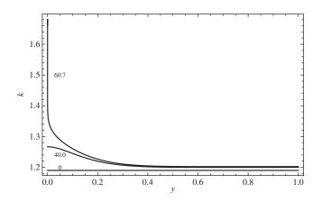
Figure 7. Spatial distribution of the work hardening parameter k for t = 0, 40 and  $60.7 \,\mu$ s.
