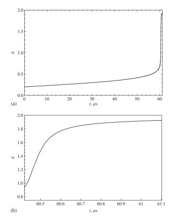
Figure 6. Time history of the temperature rise at the specimen center for (a)  $0\mu s \le t \le 61.4\mu s$  and (b)  $60.3\mu s \le t \le 61.1\mu s$ .
