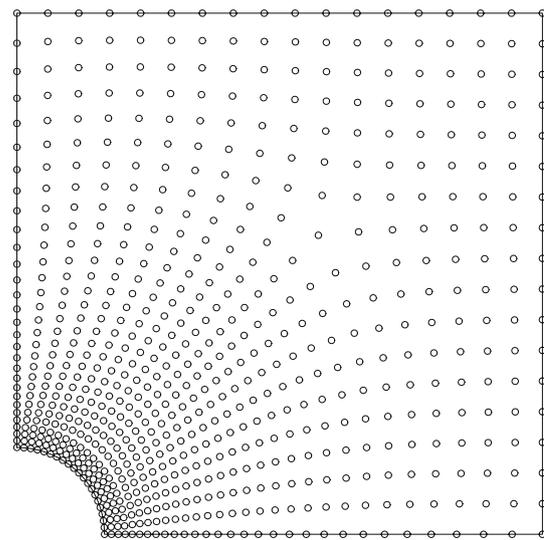
**Fig. 18** Placement of 686 particles in the domain with 21 particles on the quarter of the circle
