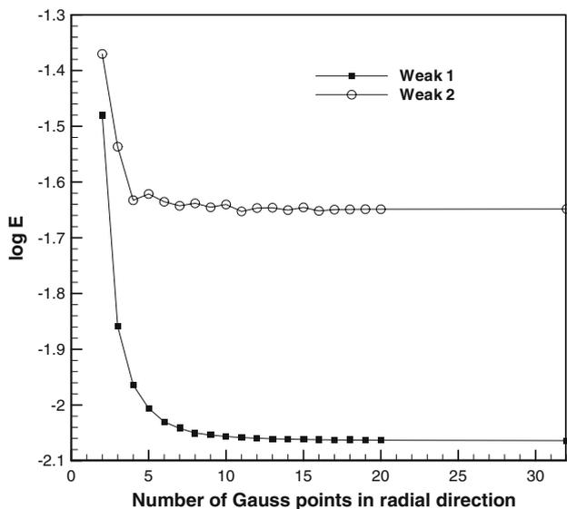
**Fig. 8** Variation of the relative error norm of displacements with the number of Gauss points in the radial direction
