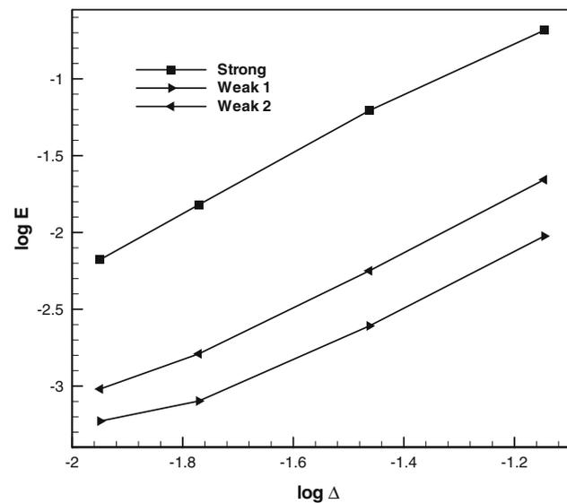
Fig. 12 Effect of the particle distance on the relative error norm of displacements computed with the strong and the two weak formulations
