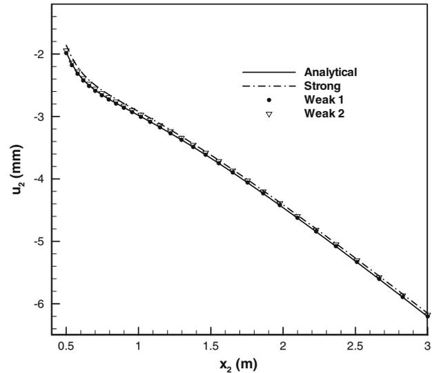
**Fig. 19** Comparison of the displacement  $u_2$  along the  $x_2$ -axis in a plate with a circular hole computed by the strong and the two weak formulations with that obtained from the analytical solution
