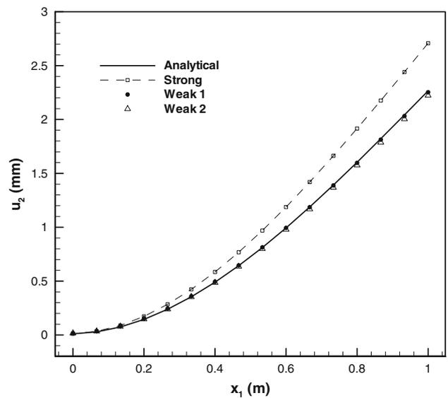
**Fig. 5** Comparison of the displacement  $u_2$  along the bottom surface of the plate computed by the strong and the two weak formulations with that obtained from the analytical solution
