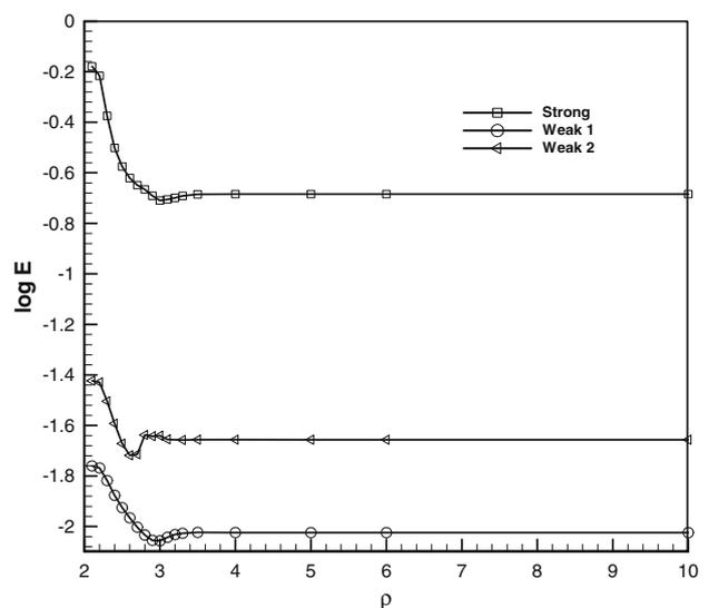
**Fig. 9** Variation of the relative error norm of displacements with the scaling factor,  $\rho$
