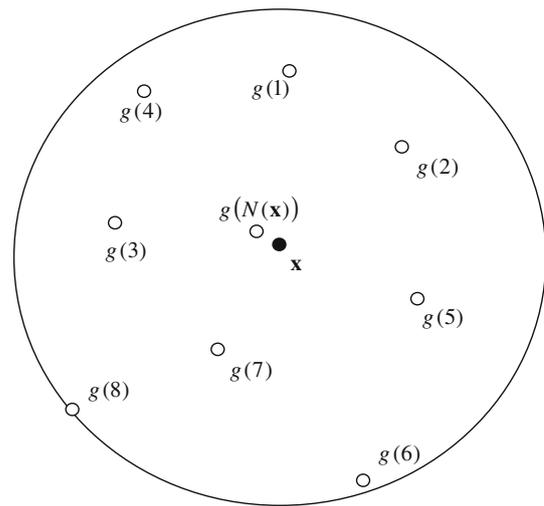
Fig. 1 Distribution of particles in the compact support of the kernel function  $W(\xi, \mathbf{x})$  associated with the point  $\mathbf{x} = (x_1, x_2, x_3)$
