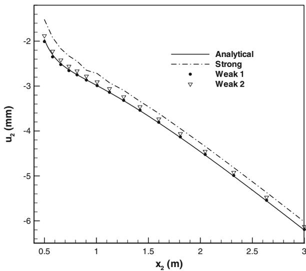
**Fig. 16** Comparison of the displacement  $u_2$  along the  $x_2$ -axis in a plate with a circular hole at its center computed by the strong and the two weak formulations with that obtained from the analytical solution
