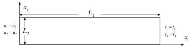
**Fig. 3** A plate subjected to prescribed displacements at the left edge and surface tractions at the right edge; the top and the bottom surfaces are traction free
