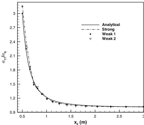
**Fig. 17** Comparison of the non-dimensional stress  $\sigma_{11}/\sigma_0$  along the  $x_2$ -axis in a plate with a circular hole computed by the strong and the two weak formulations with that obtained from the analytical solution
