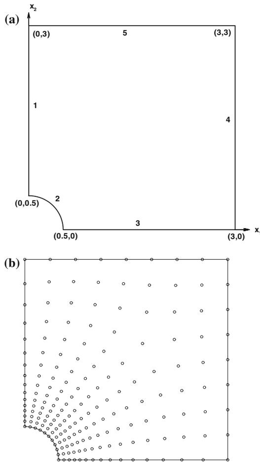
**Fig. 14** **a** Schematic sketch of a quarter of the plate used in the simulation. **b** Locations of particles in the domain studied
