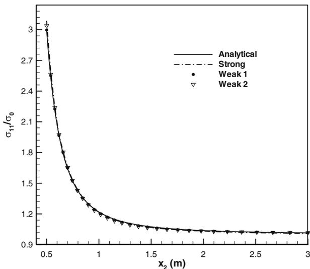
**Fig. 20** Comparison of the non-dimensional stress  $\sigma_{11}/\sigma_0$  along the  $x_2$ -axis in a plate with a circular hole computed by the strong and the two weak formulations with that obtained from the analytical solution
