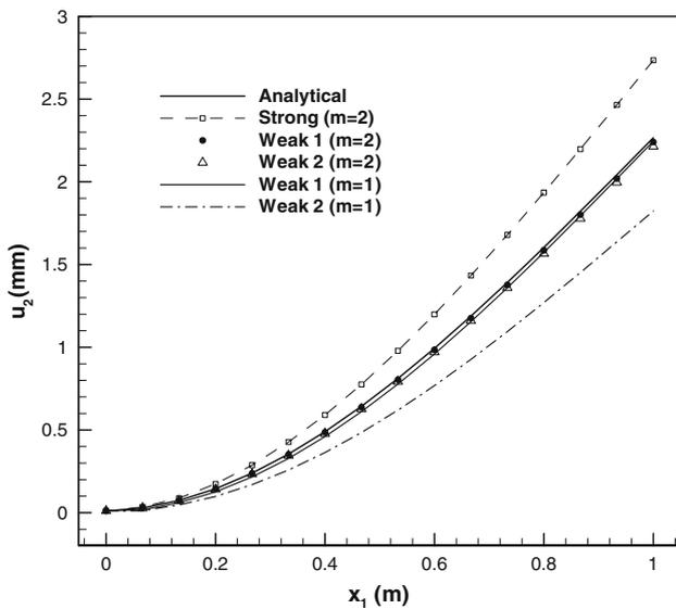
**Fig. 10** Comparison of the displacement  $u_2$  along the bottom surface for different orders ( $m = 2$  and  $m = 1$ ) of monomials used to generate SSPH basis functions
