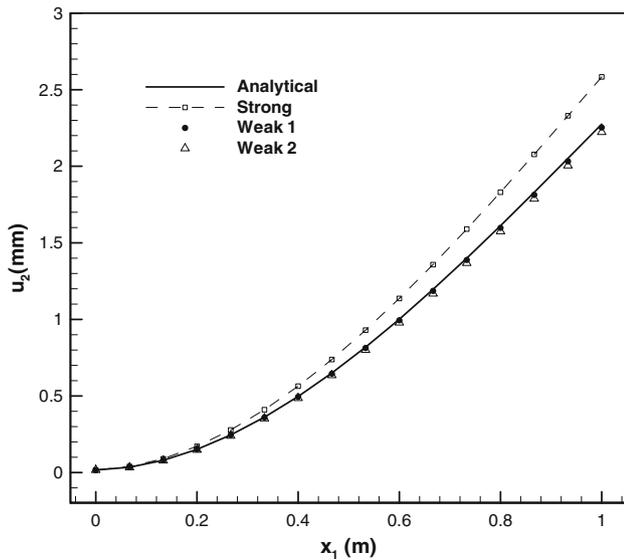
**Fig. 7** Comparison of the displacement  $u_2$  along the bottom surface of the plate computed by the strong and the two weak formulations with that obtained from the analytical solution when the Poisson ratio is increased to  $\nu = 0.499999$
