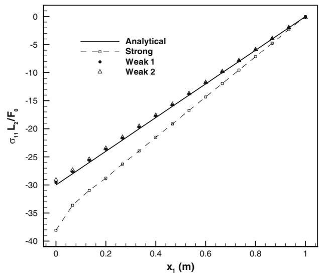
**Fig. 6** Comparison of the dimensionless stress  $\sigma_{11} L_2 / F_0$  along the top surface of the plate computed by the strong and the two weak formulations with that obtained from the analytical solution
