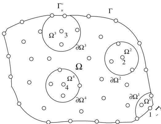
Fig. 2 Sub-domains and their boundaries for particles 1, 2, 3 and 4
