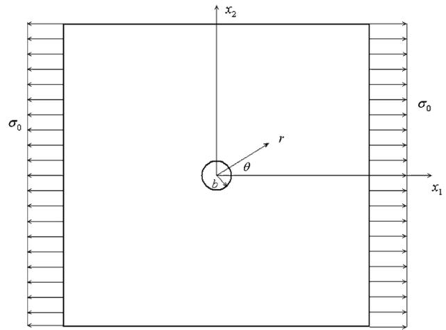
Fig. 13 Schematic sketch of a plate with a central hole and loaded in tension at two opposite edges
