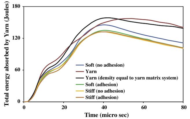
Fig. 7. Time histories of energies absorbed by the yarn. (For interpretation to colours in this figure, the reader is referred to the web version of this paper.)
