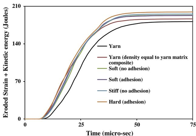
**Fig. 11.** Time history of eroded energy and the kinetic energy of the projectile for the six composite systems.
