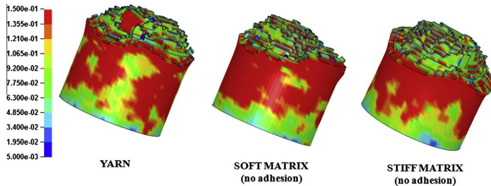
**Fig. 10.** Fringe plots of the von Mises stress (GPa) in the projectile at 100  $\mu$ s for initial projectile velocity of 450 m/s. (For interpretation to colours in this figure, the reader is referred to the web version of this paper.)
