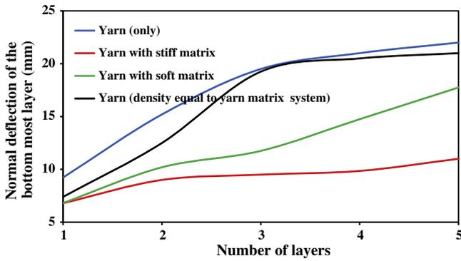
Fig. 4. Deflection of the bottom most layer vs. the number of laminate layers. (For interpretation to colours in this figure, the reader is referred to the web version of this paper.)
