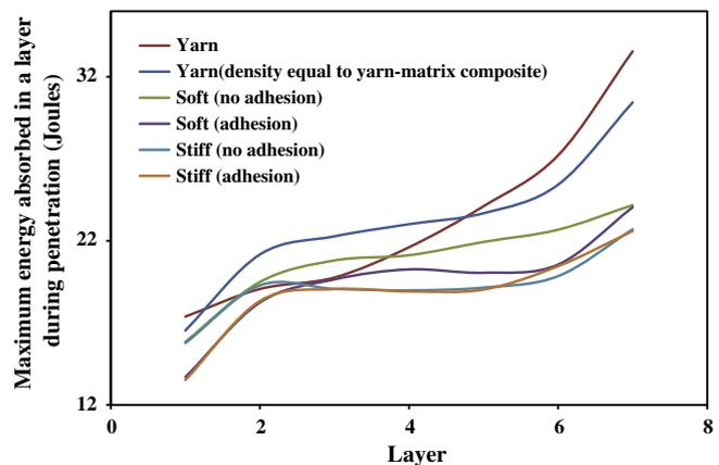
Fig. 9. Maximum energy (strain energy + kinetic energy) absorbed in each layer of the 7-layer composite. (For interpretation to colours in this figure, the reader is referred to the web version of this paper.)
