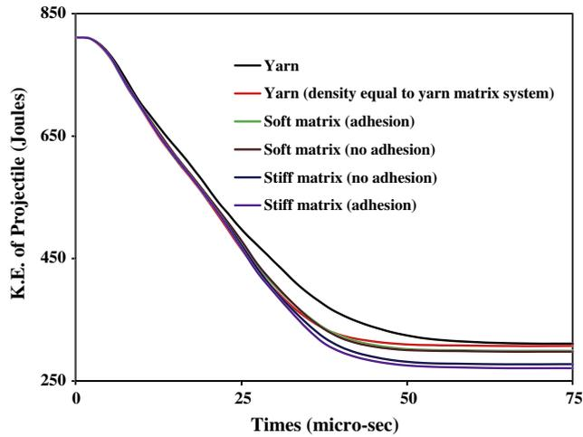
Fig. 6. Time histories of the kinetic energy of the projectile impacting the 7-layer composite laminate for impact speeds above the ballistic limit. (For interpretation to colours in this figure, the reader is referred to the web version of this paper.)
