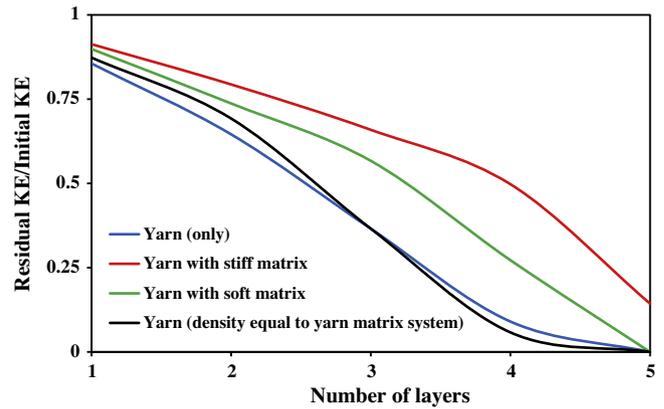
**Fig. 3.** Normalized residual kinetic energy of the projectile vs. the number of laminate layers. (For interpretation to colours in this figure, the reader is referred to the web version of this paper.)
