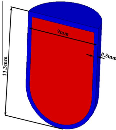
**Fig. 2.** Cross section of projectile, Remington FMJ.
