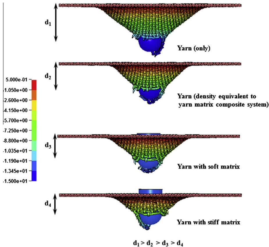
Fig. 5. Effect of matrix on the depth of the cone formed in a lamina. (For interpretation to colours in this figure, the reader is referred to the web version of this paper.)
