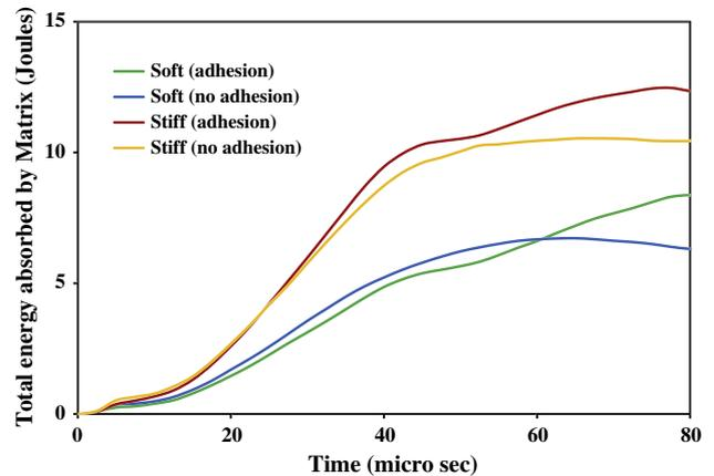
Fig. 8. Time histories of energies absorbed by the matrix. (For interpretation to colours in this figure, the reader is referred to the web version of this paper.)
