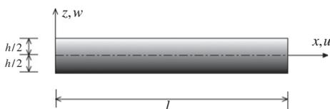
Fig. 1. Schematic sketch of a FGM beam, and coordinate axes.
