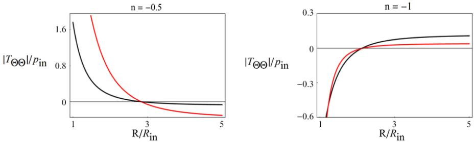
**Fig. 6** (Color online) Through the thickness variation of the hoop stress for spheres made of 1st-order (black curve) and 2nd-order elastic materials (red curve)
