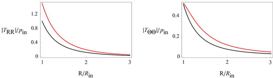
**Fig. 3** (Color online) For  $R_{ou}/R_{in} = 5$ , variation through the sphere thickness of the radial and the hoop stress magnitude for the linear (black curve) and the 2nd-order elastic materials (red curve)
