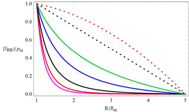
$|T_{RR}^{(1)}|$  is a monotonically decreasing function of  $R$  through the sphere thickness. For  $R_{ou}/R_{in} = 5$  we have plotted in Fig. 7  $|T_{RR}^{(1)}|$  vs.  $R$  for different values of  $n$ . It is clear that for a given value of  $R$ ,  $|T_{RR}^{(1)}|$  increases with an increase in  $n$ .
