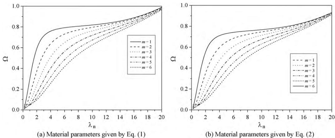
**Fig. 4.** For circumferential wave number  $m = 1, 2, \dots, 6$ , dependence of the non-dimensional frequency,  $\Omega$ , upon the parameter,  $\lambda_n$ , for the FG cylindrical shell with  $\beta = 1, \delta = 200, k = 0.1$ .
