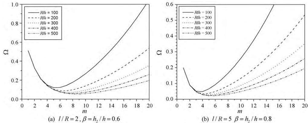
**Fig. 3.** Non-dimensional frequencies,  $\Omega$ , versus the wave number,  $m$ , for  $\delta = R/h$  ( $n = 1, k = 0.1$ ) for a FG shell with material properties given by Eq. (1).
