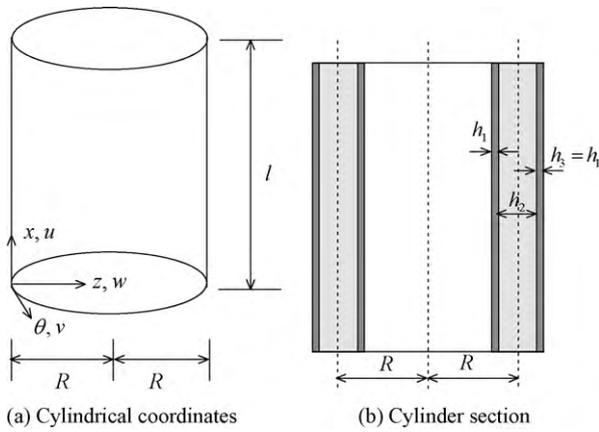
Fig. 1. Details of the geometry of the three-layer circular cylindrical shell.
