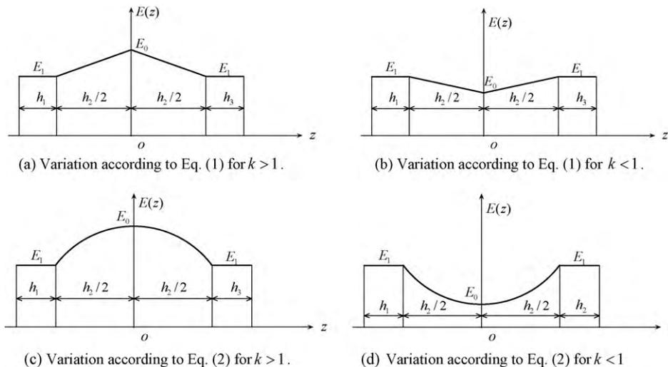
Fig. 2. Through-the-thickness variation of the elastic modulus  $E$  of the cylinder materials.
