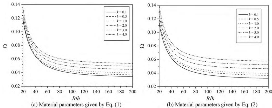
Fig. 5. Natural frequency,  $\Omega$ , versus radius-to-thickness ratio  $\delta$  for the three-layer cylindrical shell for different values of  $k$  when  $\beta = 0.6$ ,  $l/R = 5$ ,  $n = 1$ ,  $m = 1$ .
