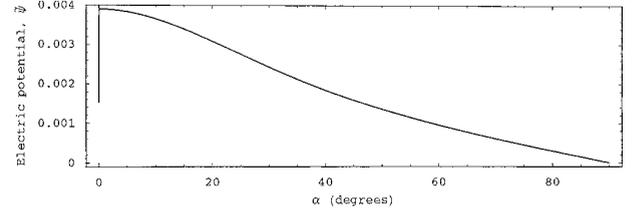
**Figure 2.** The variation with the angle  $\alpha$  of the difference in the electric potential between the end faces of a PZT5A solid cylinder subjected to pure torques at the end faces.
