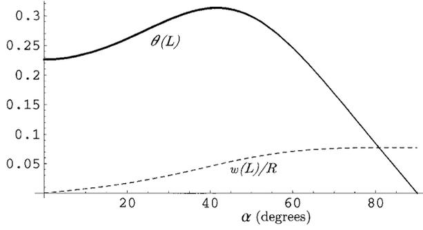
**Figure 1.** The variation with the angle  $\alpha$  of the angular twist,  $\theta(L)$ , and the normalized extension,  $w(L)/R$ , of the end  $z = L$  of a PZT5A cylindrical rod fixed at the end  $z = 0$  and subjected to a uniform charge density along its length.
