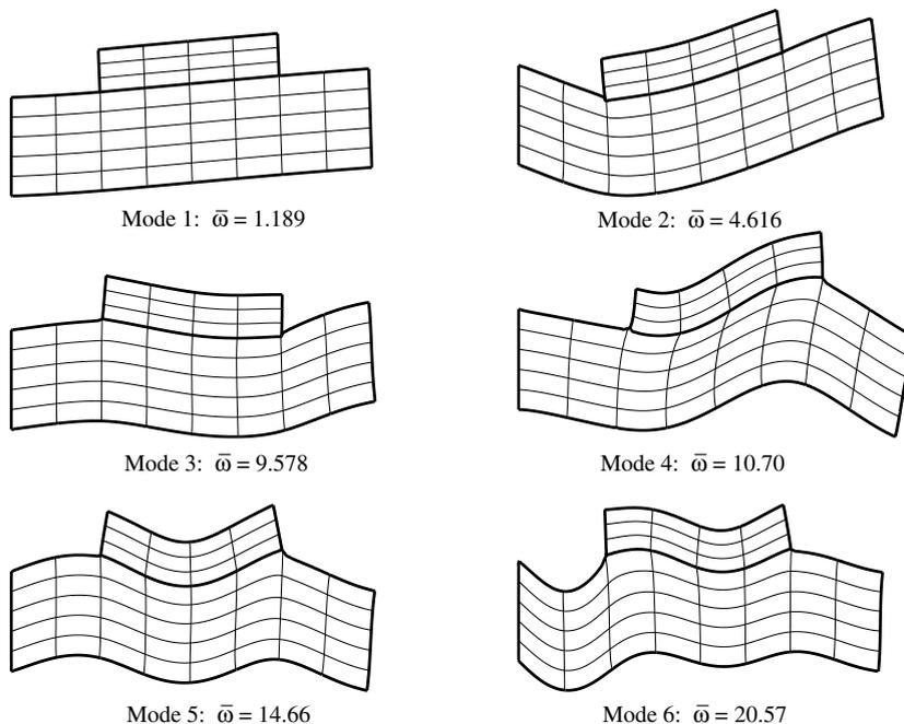
Fig. 9. The first six normalized natural frequencies and mode shapes for the graphite/epoxy cantilever plate with segmented actuator.
