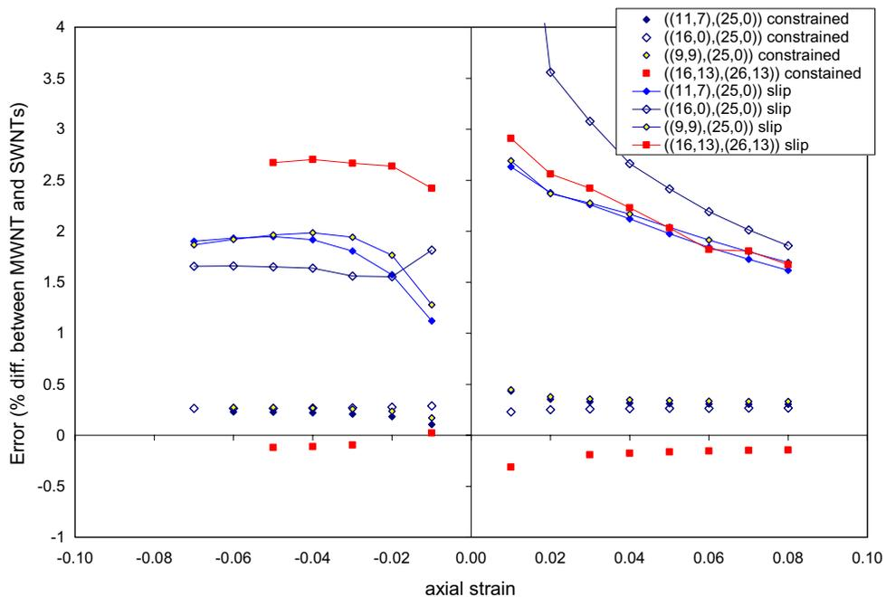
Fig. 5. Differences in strain energy/atom of a DWNT and the sum of strain energies/atom of constituent SWNTs for both fully constrained (unconnected points), and slip (solid curves) cases.
