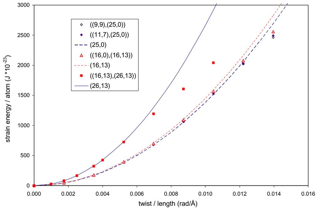
Fig. 7. Strain energy/atom for torsional deformations with loads applied only on the outer wall of DWNTs (slip condition), and SWNTs with the same atomic structures as those of the outer walls of DWNTs.
