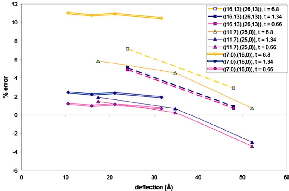
Fig. 15. Variation with the tip deflection of the percentage error in the strain energy computed by using the Euler beam theory for continuum structures equivalent to the three DWNTs. The three colors correspond to different values of the tube thickness.
