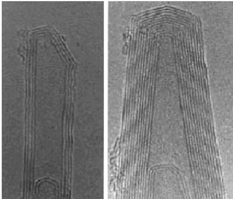
Fig. 1. TEM image of the end-cap geometry of MWNTs (from Qian et al., 2002).
