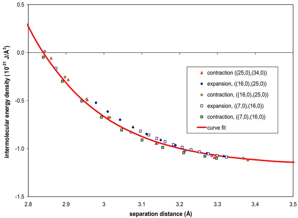
Fig. 10. Strain energy due to van der Waals force vs. distance between two adjacent walls of a DWNT; results for three DWNTs lie on the same curve.
