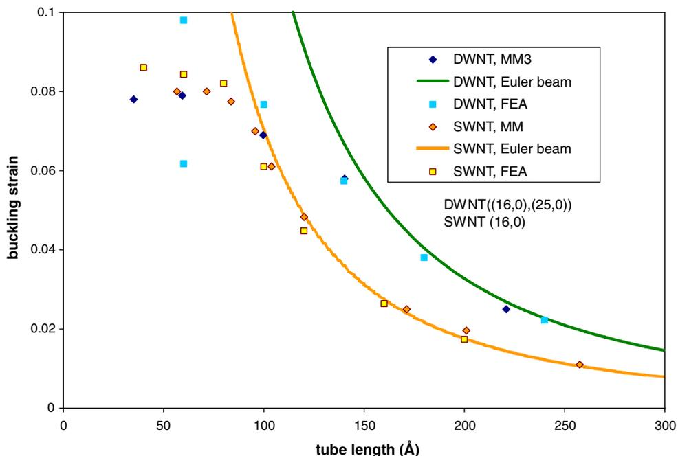
Fig. 16. Variation with the tube length of the axial strain at buckling for two differently structures DWNTs, their constituent SWNTs, and that predicted by the Euler buckling theory and FEA by using the equivalent continuum model.
