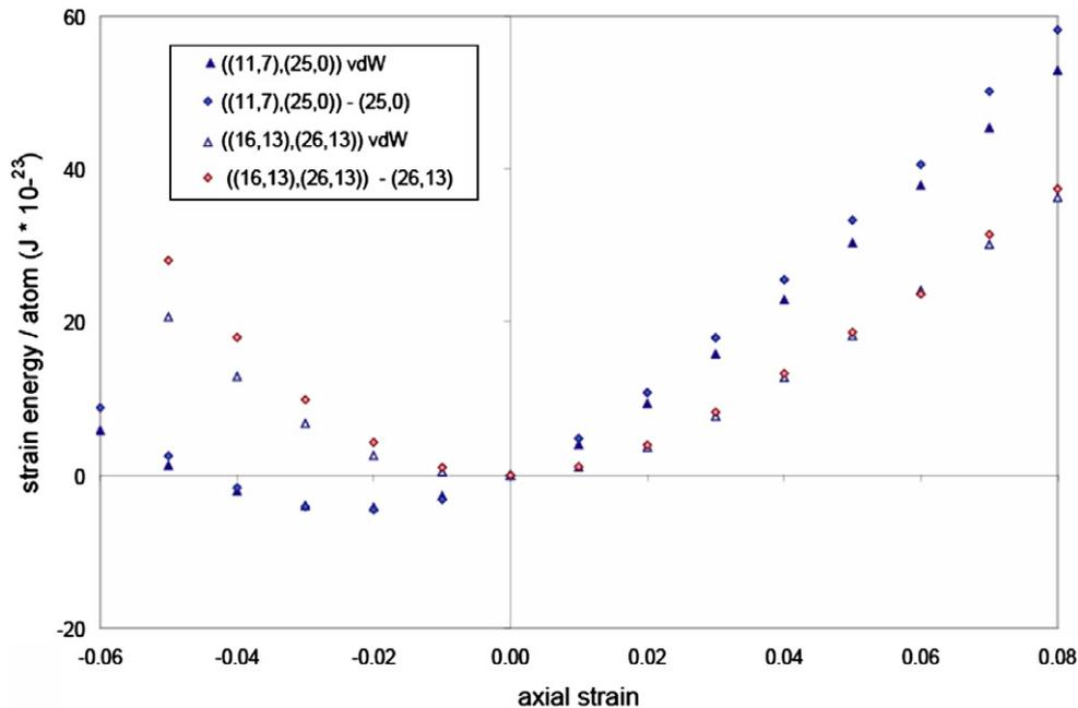
Fig. 6. For two DWNTs, comparison of strain energy due to intermolecular van der Waals forces and the difference in strain energies of a DWNT loaded under slip conditions and identically loaded constituent SWNT.
