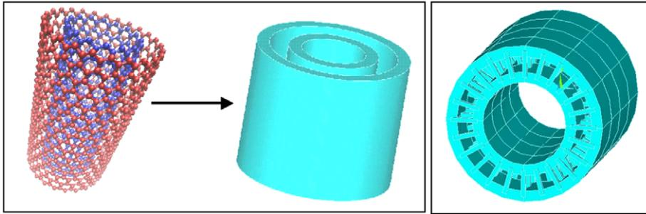
Fig. 12. Left, a continuum structure equivalent to a DWNT; right, a cross-section showing trusses connecting the two concentric tubes to account for van der Waals force.
