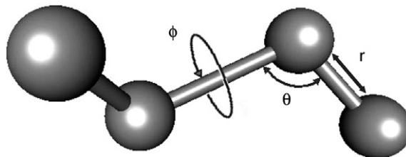
Fig. 2. Definitions of variables  $r$ ,  $\theta$  and  $\phi$  used in defining pair-wise MM3 potentials.
