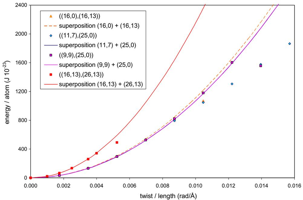
Fig. 8. Strain energy/atom for torsional deformations of fully constrained DWNTs and that obtained by adding the strain energy/atom of their constituent SWNTs.
