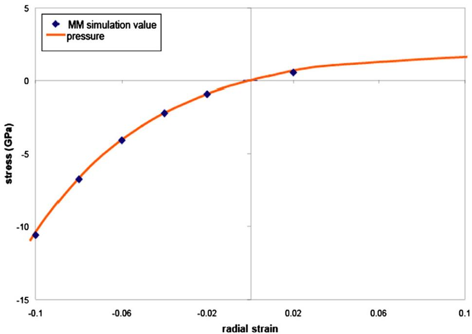
Fig. 11. Radial pressure vs. radial strain derived from MM simulations of radial expansion/contraction of a wall of a nanotube.
