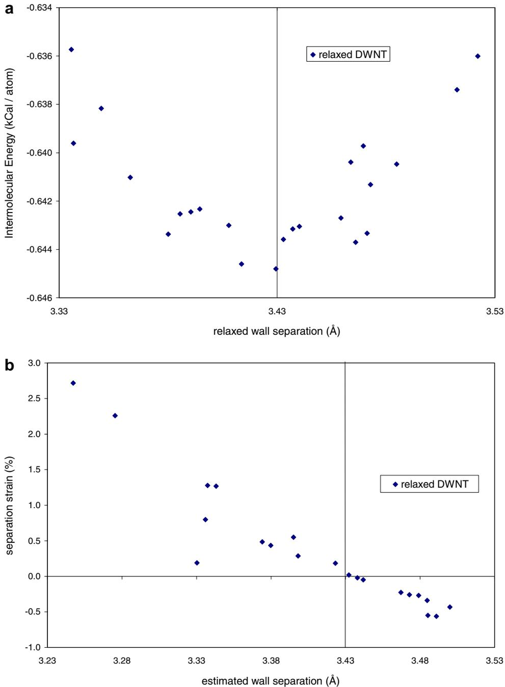
Fig. 3. For DWNTs, (a) intermolecular energy vs. wall separation distance, and (b) the separation strain vs. the initial distance between walls of relaxed SWNTs constituting the DWNT.
