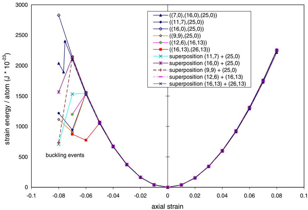
Fig. 4. For axial deformations, strain energy of a fully constrained DWNT vs. axial strain, and sum of strain energies of the constituent SWNTs vs. axial strain.
