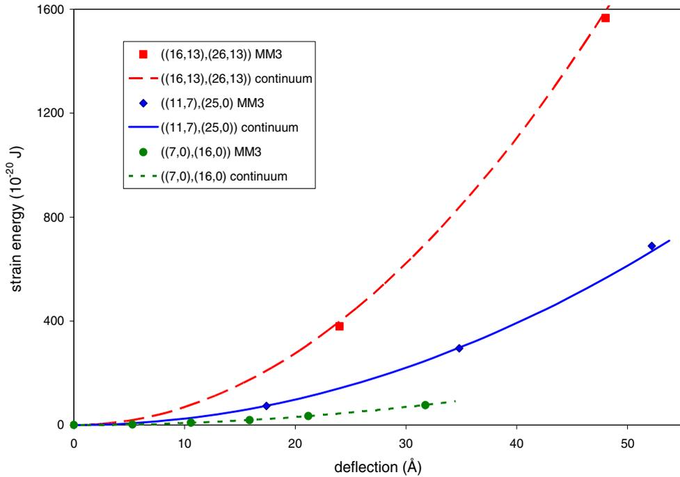
Fig. 14. Strain energies of cantilever DWNTs with a point load at the unclamped end computed by MM simulations and the Euler beam theory using the equivalent continuum model.
