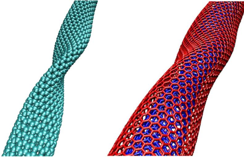
Fig. 9. Buckled shapes of (16,0) SWNT, and ((16,0),(25,0)) DWNT under torsional loads.
