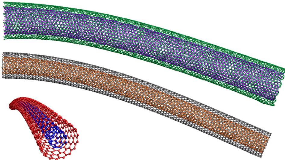
Fig. 13. Deformed configurations of three cantilever DWNTs loaded by a point load at the free end.
