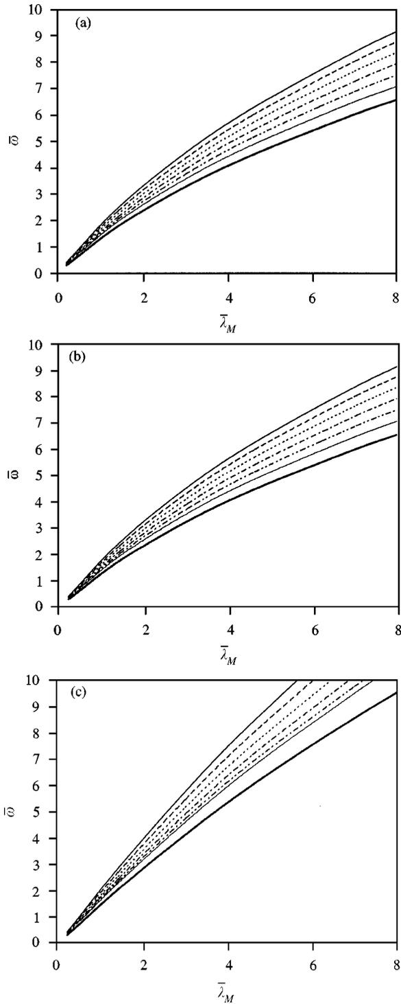
Figure 3. Natural vibration frequency of the dominant flexural mode versus the membrane eigenvalue when using (a) the third order theory, (b) the first order theory, and (c) the classical theory for the plate: —, ceramic; ---,  $n = 0.2$ ; - - - - ,  $n = 0.5$ ; - · - · - ,  $n = 1$ ; - · - - - ,  $n = 2$ ; — — — — ,  $n = 5$ ; ———, metal.
