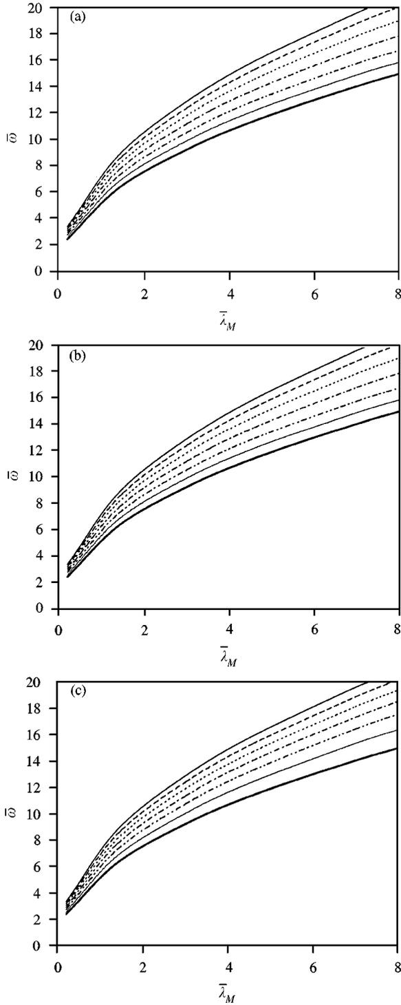
Figure 4. Natural vibration frequency of the dominant stretching mode versus the membrane eigenvalue when using (a) the third order theory, (b) the first order theory, and (c) the classical theory for the plate: —, ceramic; ---,  $n = 0.2$ ; - · - ·,  $n = 0.5$ ; - - - -,  $n = 1$ ; - · - · - ·,  $n = 2$ ; — — — —,  $n = 5$ ; ———, metal.
