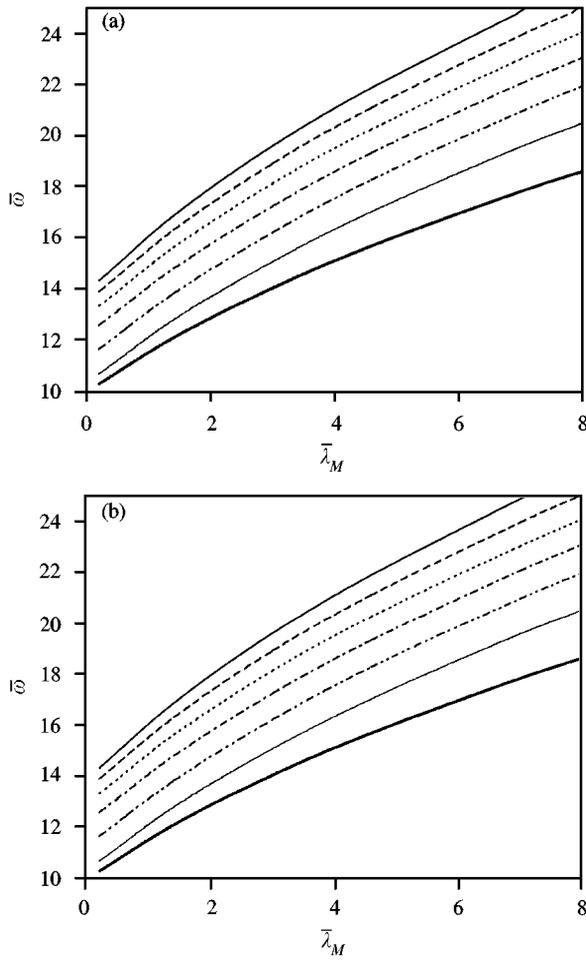
Figure 5. Natural vibration frequency of the dominant thickness-shear mode versus the membrane eigenvalue when using (a) the third order theory, and (b) the first order theory for the plate: —, ceramic; - - -,  $n = 0.2$ ; - · - · -,  $n = 0.5$ ; - - - - -,  $n = 1$ ; - · - · - · -,  $n = 2$ ; ———,  $n = 5$ ; ———, metal.
