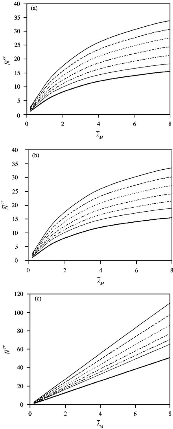
Figure 2. Critical buckling load versus the membrane eigenvalue when using (a) the third order theory, (b) the first order theory, and (c) the classical theory for the plate: —, ceramic; ---,  $n = 0.2$ ; - · - ·,  $n = 0.5$ ; - - - -,  $n = 1$ ; - - - -,  $n = 2$ ; —,  $n = 5$ ; —, metal.
