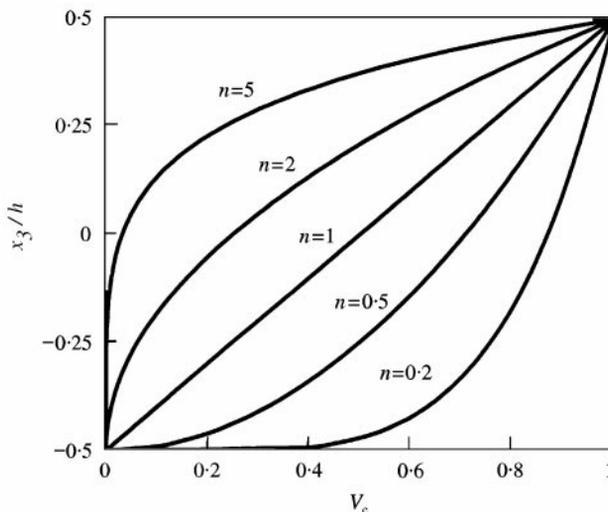
Figure 1. Through-the-thickness distribution of the volume fraction of the ceramic.
