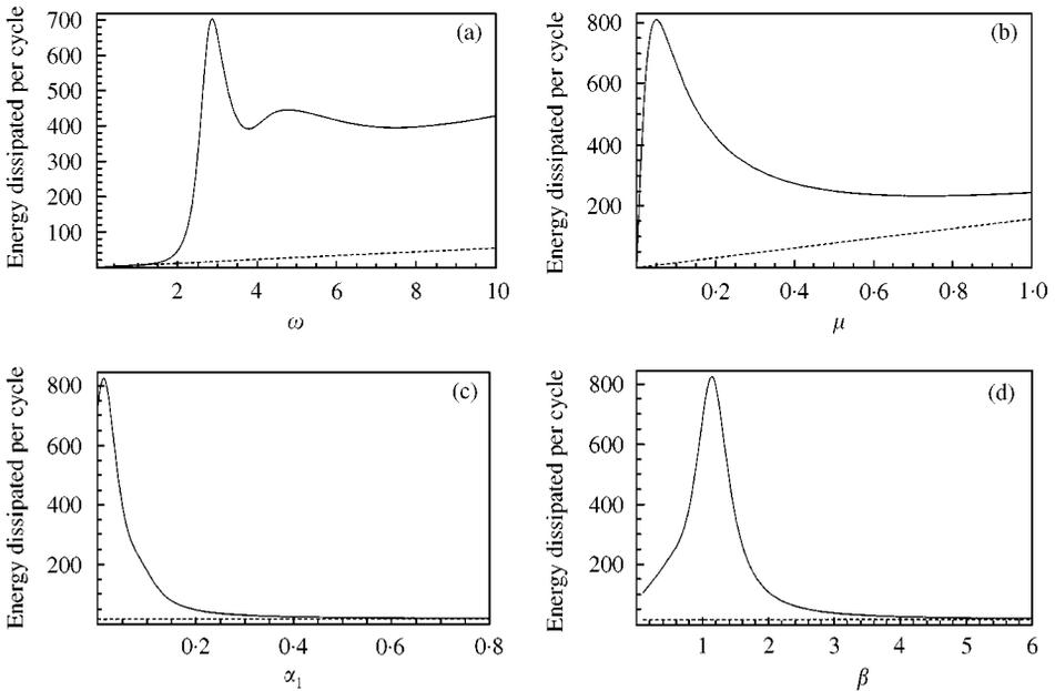
Figure 3. The dependence of the energy dissipated per cycle per unit cylinder length,  $\Psi$ , upon (a) the frequency  $\omega$ , (b) the Newtonian viscosity  $\mu$ , (c) the higher order viscosity  $\alpha_1$  and (d) the elastic modulus  $\beta$ : (—), with inertia; (- - - -), without inertia.
